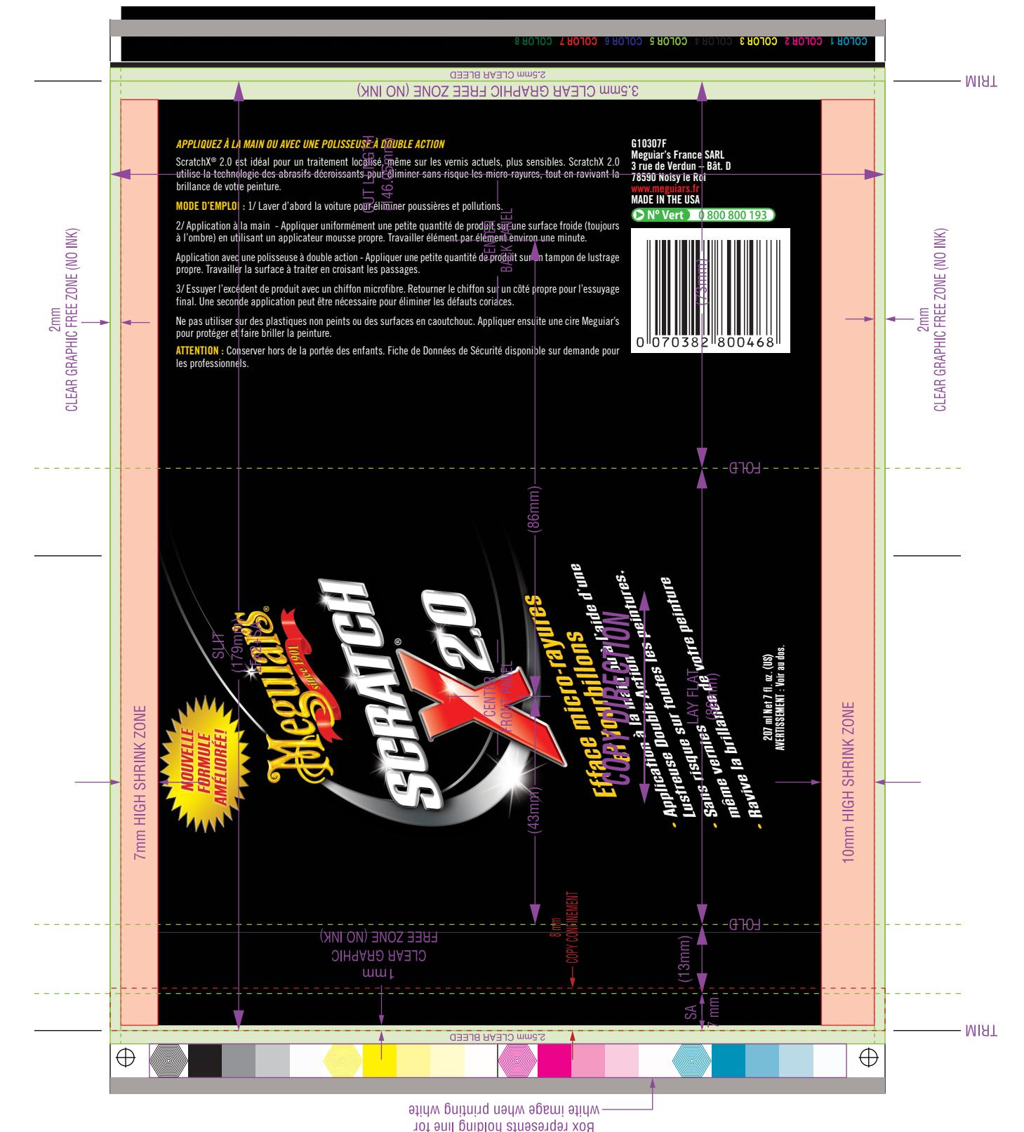
146.05mm Cut Length x 86mm Lay Flat (+1mm/-0) Sli'e (Lfx2+SA) = 179mm
