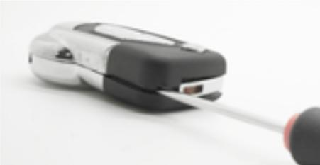
DÉBOÎTEZ LA COQUE À L'AIDE D'UN TOURNEVIS PLAT. RÉCUPÉREZ LA PILE, LE CIRCUIT ÉLECTRONIQUE AVEC SON TRANSPONDEUR EN LE SAISISANT PAR LES BORDS POUR ÉVITER TOUT CONTACT AVEC LA SURFACE.
