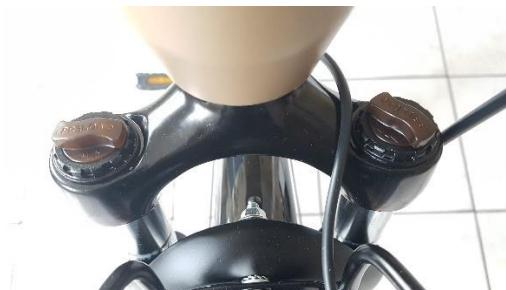
Your fork is equipped with a preload adjustment, turn the knobs clockwise to lightly harden your suspension.
