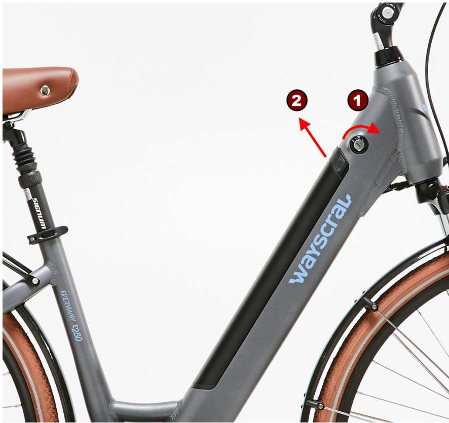
To replace the battery, insert it starting at the bottom and then rotate the top until it is properly clipped in
