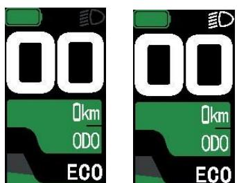
Your display is also backlit. The screen brightness can be adjusted by holding down the "i" button for 2 seconds.
