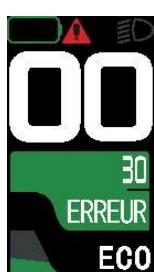
When an error code appears on the display, the "⚠" icon appears on the screen.
