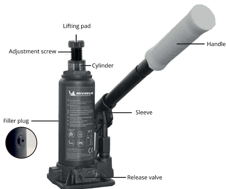
Figure 1 Hydraulic bottle jack components
