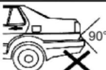
Be sure no other parts of the vehicle falls into the detecting range of the sensors so as to avoid false detection.
