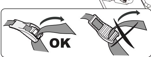
**B/ INSTALLATION DES SANGLES DE SECURITE / INSTALLATIE VAN VEILIGHEIDSSPANRIEMEN /
