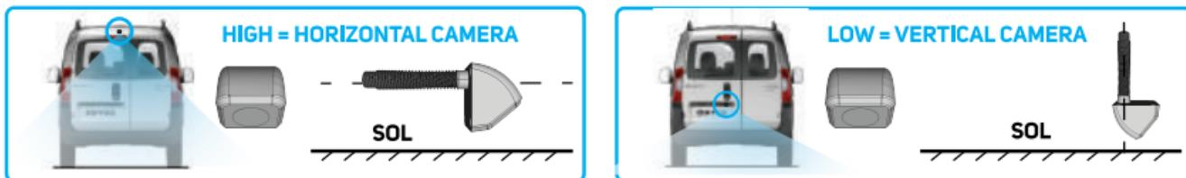
Withdraw the night light of plate of its housing to locate the most adequate site. In the trunk, locate how to bring out the wire of the camera, to allow the fixing of the camera and to be able to connect it on the sons of origin of the vehicle as indicated previous pages.
