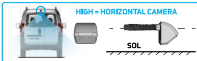
Remove the trimming from your trunk in order to locate how to bring out the wire of the camera and to allow the fixing of this one.
