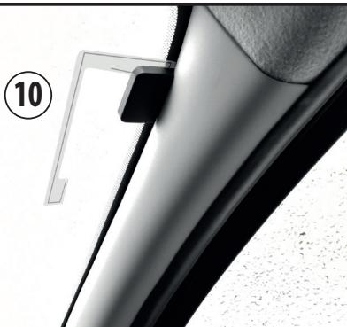
Install the DAB+ antenna on the right-hand side of the windscreen, ensuring the bronze section touches the vehicle's frame (this is necessary to power the antenna).
