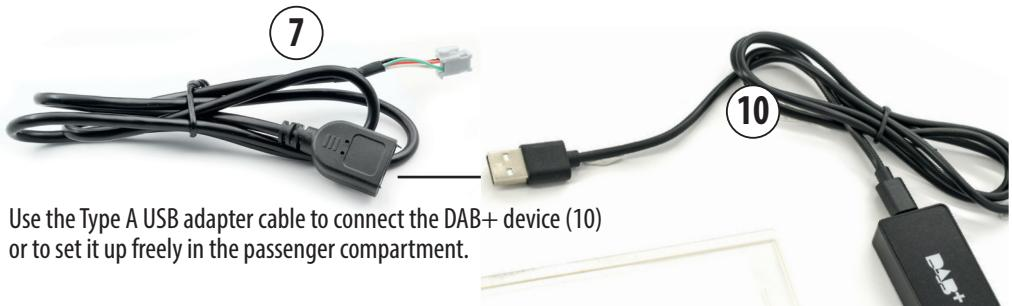
Use the Type A USB adapter cable to connect the DAB+ device (10) or to set it up freely in the passenger compartment.
