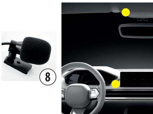
Find the best spot to place the microphone (7) inside the vehicle, making sure it faces and is near the driver for optimum performance.
